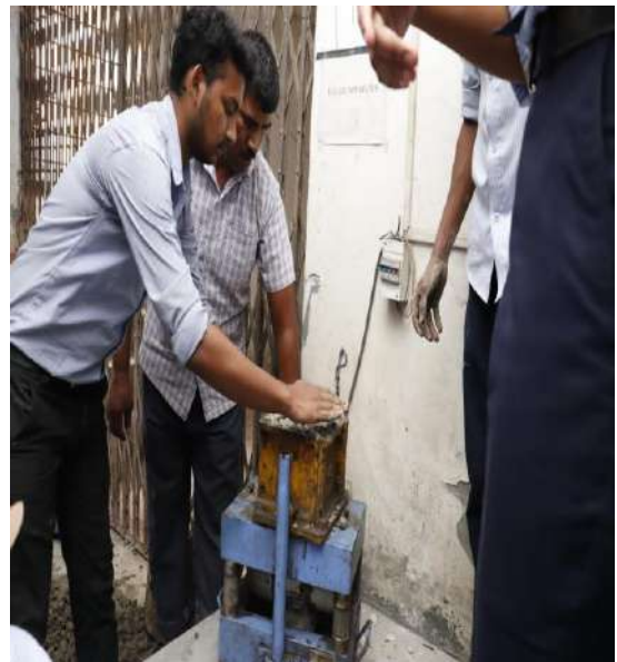
Concrete cube are extracted
