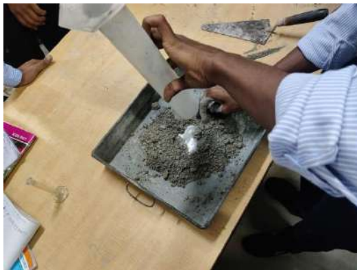
Water is mixing with cement for conducting Penetration Test
