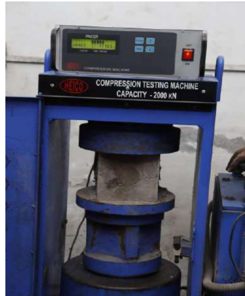
Compressive strength test
