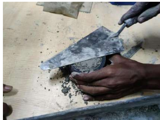
Cement paste put in the mould
